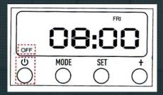
b. Long press to for 2 seconds to turn the power on, the screen will display ON.
